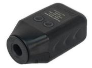
AC 03 sound calibrator is suitable for sound pressure calibration of sound level meters and other sound measurement equipment. The sound calibrator has a built-in feedback microphone to ensure a highly stable sound pressure output. 94db SPL or 114 dB SPL dual sound pressure levels is optional, which can make a calibration even in noisy environment. 1 inch, 1/2 inch and 1/4 inch microphones can be calibrated with 1kHz calibration frequency.
